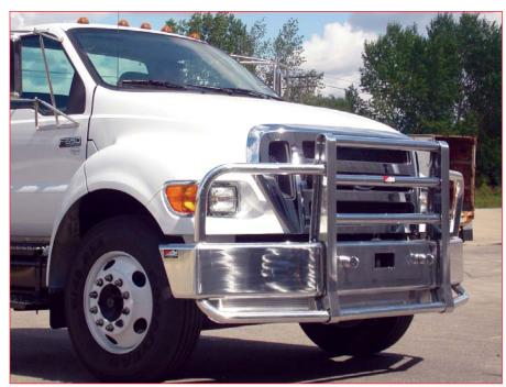
\*  $\frac{1}{2}$  extruded bumper with 2  $\frac{1}{2}$  tubing &  $\frac{1}{4}$  wall thickness, integrated tow hitch with easy access tilt system.
